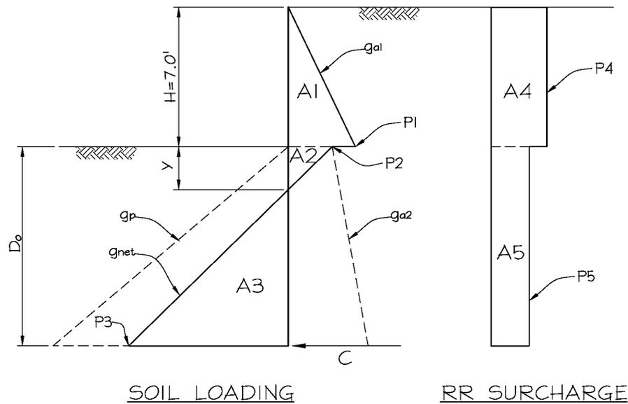
$$g_{a1} = 30(\text{PILE SPACING}) = 30(8) = \underline{240 \text{ psf}}$$
