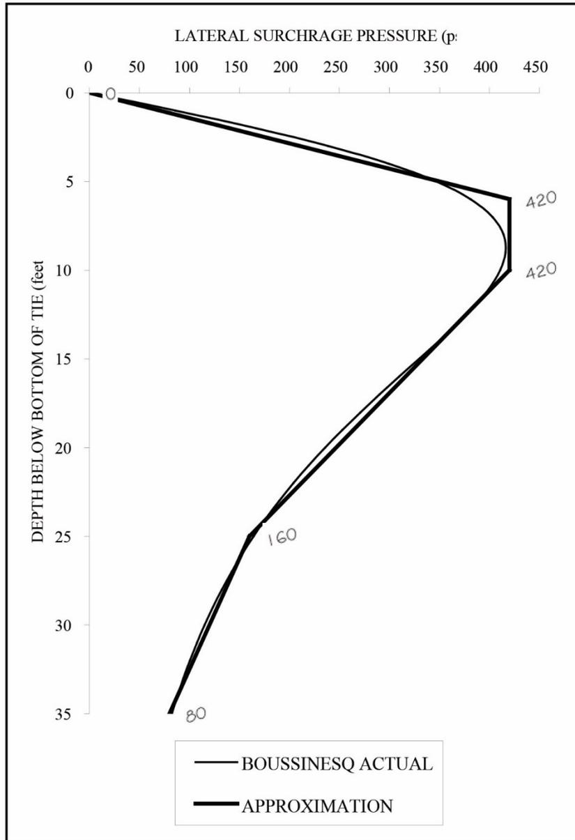
ANALYZE SHORING WALL USING BEAM ANALYSIS SOFTWARE TO DETERMINE DEPTH OF EMBEDMENT REQUIRED FOR STABILITY (I.E., SUM OF MOMENTS ABOUT BRACING LEVEL EQUAL TO ZERO).
