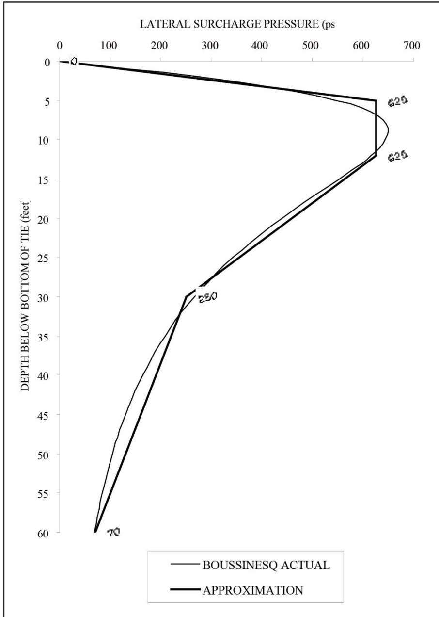
ANALYZE SHORING WALL USING BEAM ANALYSIS SOFTWARE TO DETERMINE DEPTH OF EMBEDMENT REQUIRED FOR STABILITY (I.E., BALANCE MOMENTS DUE TO LOADS ACTING BELOW THE LOWEST BRACING LEVEL).
